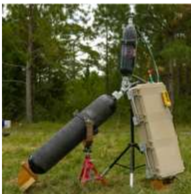
The prototype Hydrogen Tactical Refueling Point (H-TaRP). (Photo: USMC/Lance Cpl Cheyenne Stillion) (The Shephard News Team, 2022)
