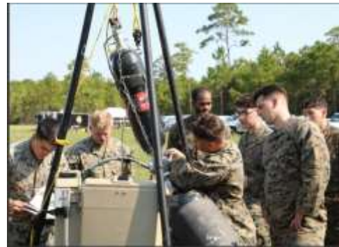
The H-TaRP prototype is demonstrated at Camp Lejeune, N.C. H-TaRP is designed to provide power to forces in expeditionary environments by combining water with aluminum to create hydrogen fuel. (U.S. Navy photo by David Taylor) (Hochenberg, 2022)
