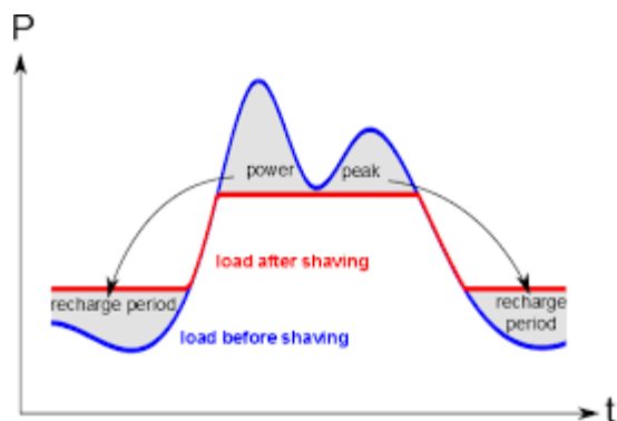
Figur 2: Prinsippet bak peak shaving.
