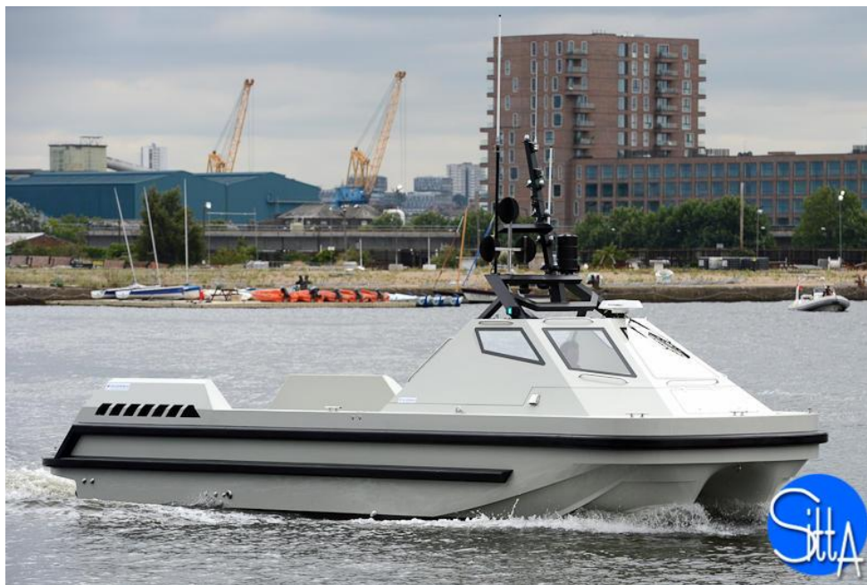
Figur 26: ARCIMS (Naval Technolgy, u.å., ATLAS Remote Combined Influence Minesweeping System (ARCIMS))
