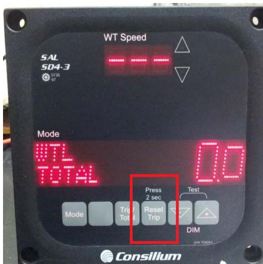
Fig. 6. HMI electromagnetic log, reset trip button highlighted in red
