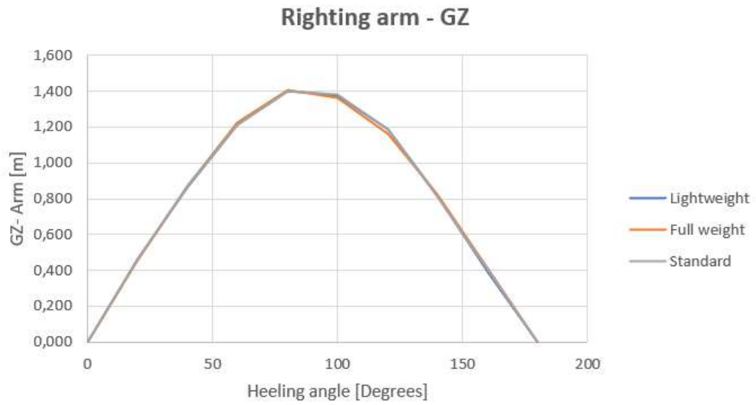
Figure 9: Heeling angle and positive GZ
