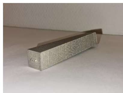
Figure 4.2-3 Warpage in specimen 3 seen from the side
