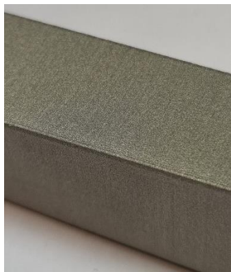
Figure 4.2-4 Sideview of specimen 3 after sintering
