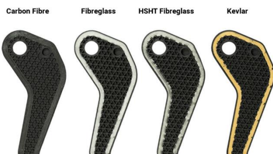
Figure 5.2-1 Different reinforcements done by Markforged (Ziółkowski & Dyl, 2020)
