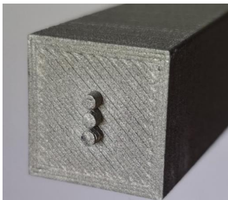
Figure 4.2-5 Upper cross section of specimen 3 after sintering
