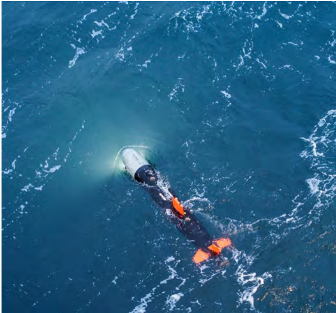
Autonomous Undersea Vehicle, SeaCat, conducting maneuvers in the North Sea.
