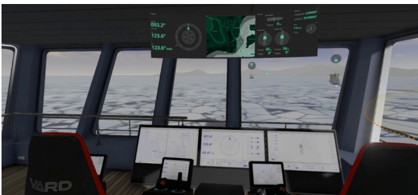
Fig. 5. Screenshot from a VR-based simulator used to prototype and test AR applications. Credit: OICL.
