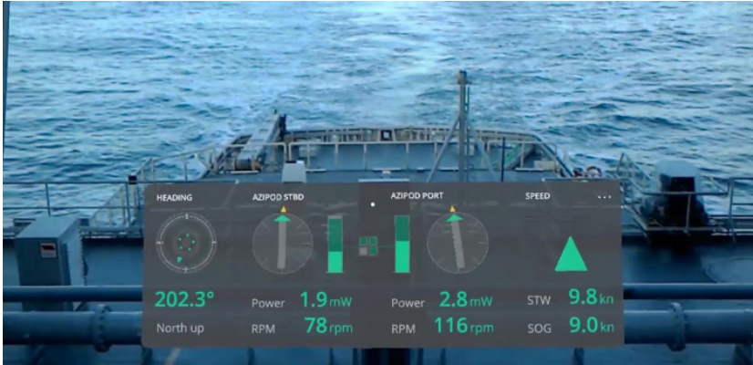
Fig. 4. Maritime functions rendered in AR, from left to right: heading information from a compass, power information about azipod thrusters, and speed. Credit: OICL.
