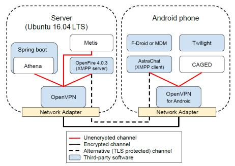
Figure 8: Server and Android phone deployment for experiments.
