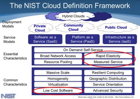
Figure 4: The NIST Cloud Definition Framework<sup>16</sup> with added highlighting.
