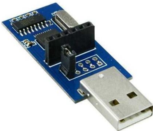
Figur 104: DAC23 USB til RS232 konverter. Kilde: https://www.matiot.com/usb-to-rs232-converter-dac13
