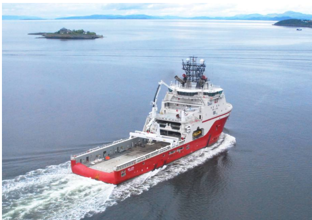
In September 2019, the AHTS Boa Jarl and her sister ship were hired to serve with the Norwegian Coast Guard for five years. The ships are 91 meters long, 22 meters wide and can carry a load of 3790t. They have a deck area of 828 square meters, max deck load is 1600 tons, deck strength is up to 15 tons per square meters. Photo: Skipsrevyen.
