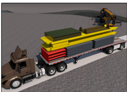
The Tec-Trans container based Smartbridge is 20-32 meters long, 4 meters wide and built for loads over 100 tons. Photo: Tec-Trans
