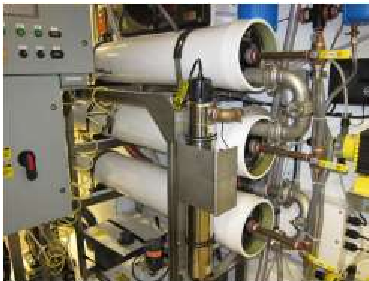
Figur 12: Tre RO- membraner i SWRS (Headquarters, Department of the Army, 2016).
