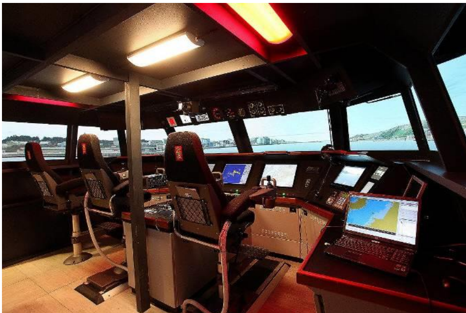
Figure 7-3: Type specific 1:1 simulator for Skjold Class (courtesy NNC)
