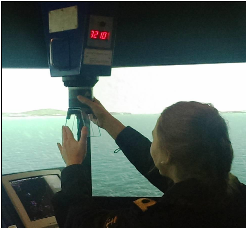
Figure 3-1: Optical Bearing Device (OBD) integrated in IBS (courtesy NNC)
