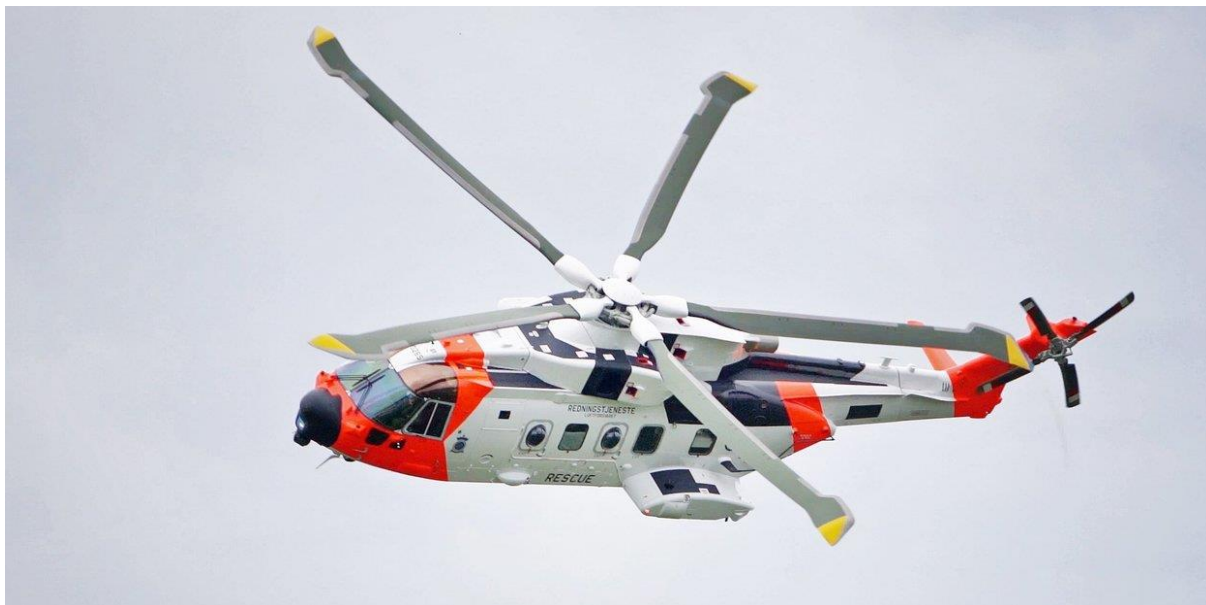
Figur 5 Norwegian All Weather Search and Rescue Helicopter AW101 (Foto: Eirik Helland Urke)
