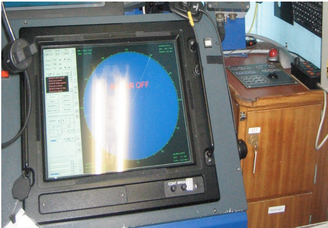
Figure 5-1: The radar screen (left) and the operator panel with tracker ball (to the right).
