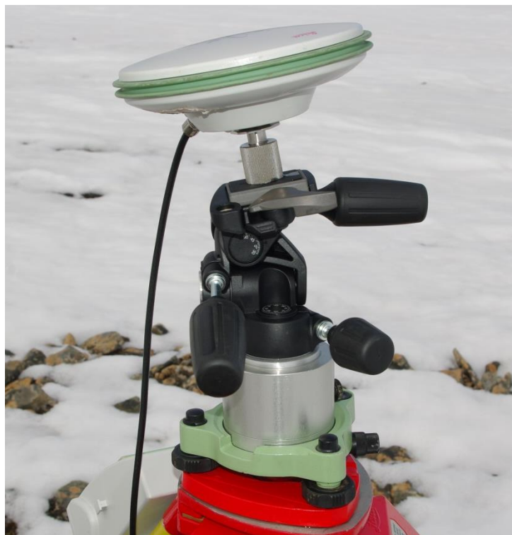
Figure 3.3 Rover Station Manfrotto tilted 15 Degrees to West before the measurements started.
