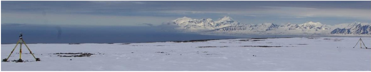
Figure 3.7 Photo of rover station to the left and base station to the right at Svalbard Satellite Station at the beginning of the measurements
