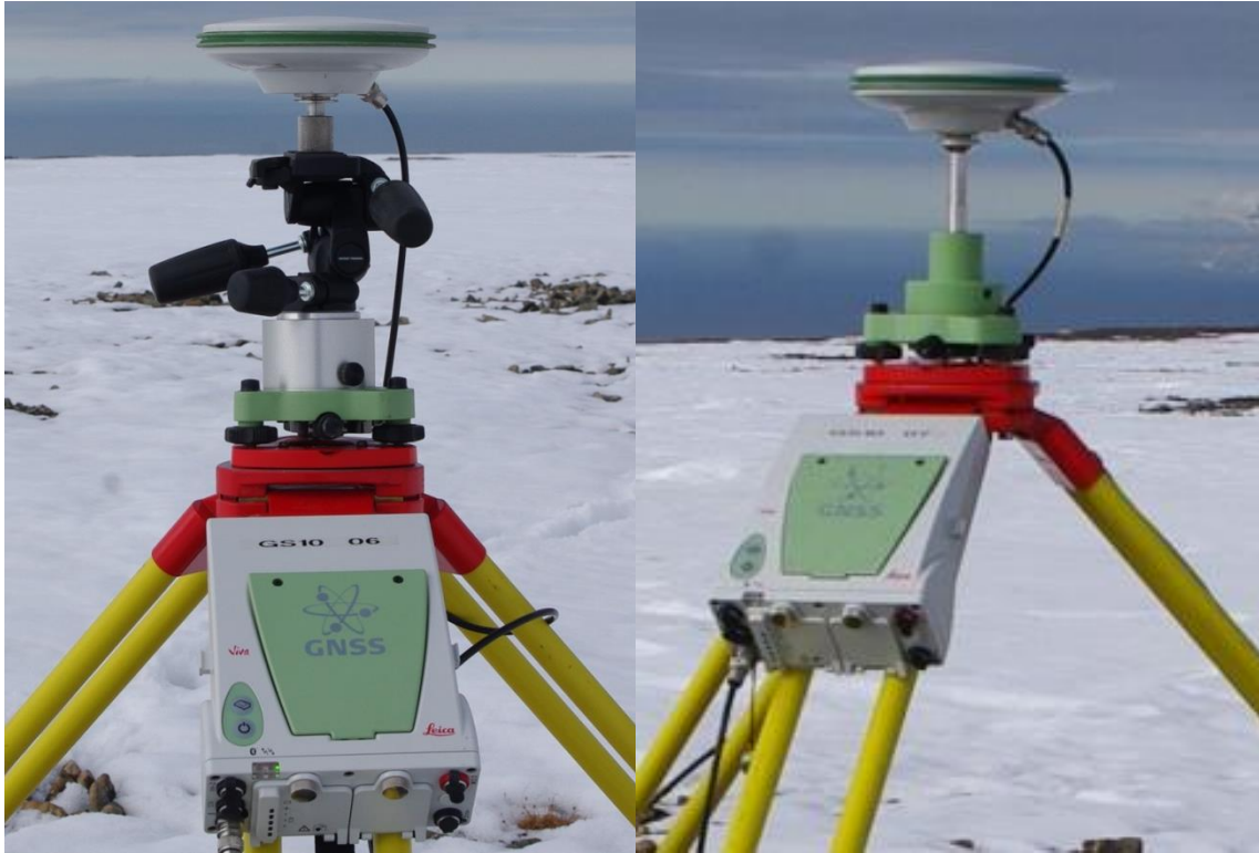
Figure 3.1 Photo at Svalbard of the rover station with the Manfrotto tilt head and screw transitions to the left and the base station to the right.
